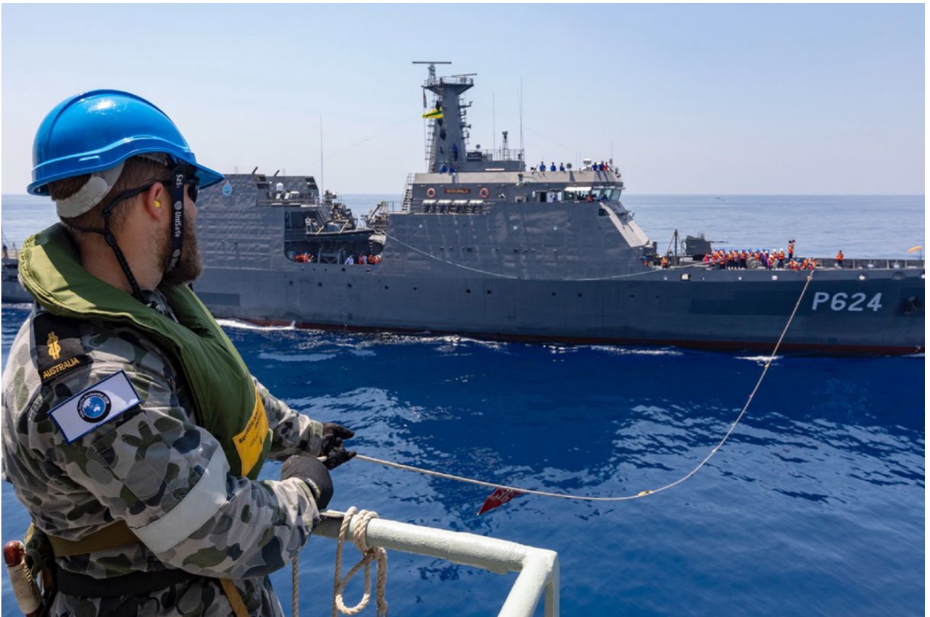
Source: Royal Australian Navy sailor Able Seaman Boatswains Mate Taylor Bootle manages the distance line during a Replenishment at Sea Approach (RASAP) exercise with Sri Lanka Navy Ship Sindurala as part of Indo-Pacific Endeavour 2019, Department of Defence image library.
